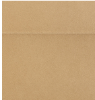
Long sealing seam: prone to leaks and dust build-up at the open valve end
